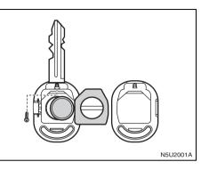
To replace the battery in the remote keyless entry transmitter, do the following:
